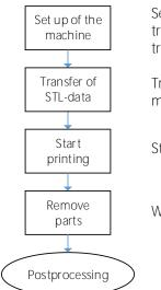
Setup machine for the resin (Settings see machine manual) and fill the polymer tray/basement. To avoid impurities, resin mixes and contamination a separate polymer tray/basement must be used.
