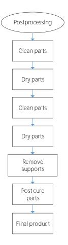
Cleaning in 2-propanol (min. >96 %) (max. 5 minutes); Cleaning under pouring conditions (no ultrasonic); Recommendation: Magnetic stirrer with bar or lab shaker. Clean and rinse gaps separately.
